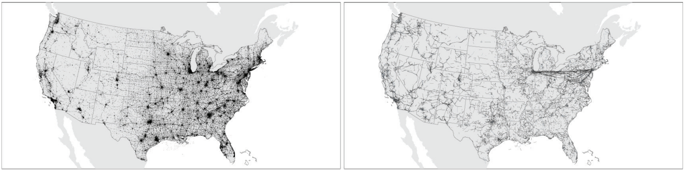
FIG. 11: A map of 93,600 paths present in 187,338 microwave site-based license applications for the two years prior to September 1, 2012 (left) and of 191,290 towers culled from the FCC database (right). Colors indicate frequency bands: 6 GHz (black), 11 GHz (charcoal), 18 GHz (dark gray), and other (slate gray).
