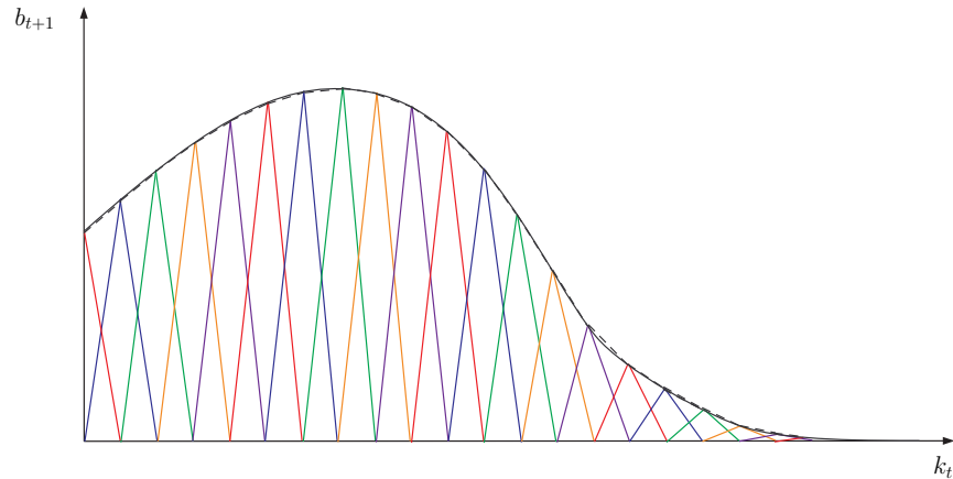
Figure 9: Finite Element Approximation
